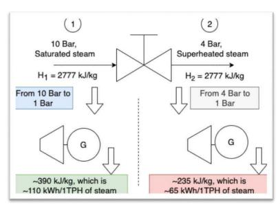
the 4 Bar steam after the PRV can only produce 65 units as the PRV has destroyed the ability of steam to produce power. Hence instead of the PRV, an energy recovery system could be used to improve efficiency of the process.
