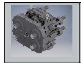
Phoenix Field Trial – Pilot batch: Specifications Rated power: 18.5 kW Pressure range: 10.5 Barg to 3 Barg Flow rate: up to 0.6 TPH RPM: 3000 Cost of pilot ~ 15 to 18 Lakhs Typical payback: < 18 months, depends on cost of electricity saved
